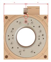
necessary. For the alignment of the rotor flange, a single bore Ø4H6 with aligned marking on the shaft and a marking on the symmetry axis of the housing is provided. The absolute zero point is in straight alignment of the two markings.
