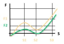
The patented function "IForce Calibration" is able to compensate the magnetic cogging forces, the load and the friction forces of the ROTAX® Rxhq direct drive in a very simple way. This makes it possible to limit and monitor torques in processes. Together with the XENAX® servo controller, complete torque/displacement diagrams can also be recorded an additional sensor is not necessary.
